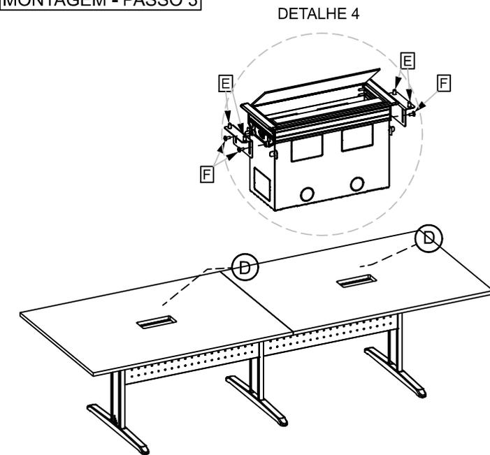
PARA FINALIZAR A MONTAGEM, PEGUE A CAIXA BASIC (D) E DESTAQUE AS ABAS LATERAIS CONFORME DETALHE 4, PARA QUE A MESMA POSSA SER FIXADA NA MESA.
